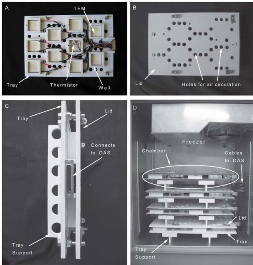
**Figure 1** Layout and design of the chambers used for cold-hardiness evaluation. Each chamber consists of (A) a tray with 10 wells containing thermoelectric modules (TEM), where four to five buds or two to three cane pieces are placed and (B) a lid that when tightened ensures close contact between sample and TEM. The data acquisition system (DAS) is connected to (C) the cold-hardiness chamber in the freezer, where up to four chambers (D) can be run simultaneously.
